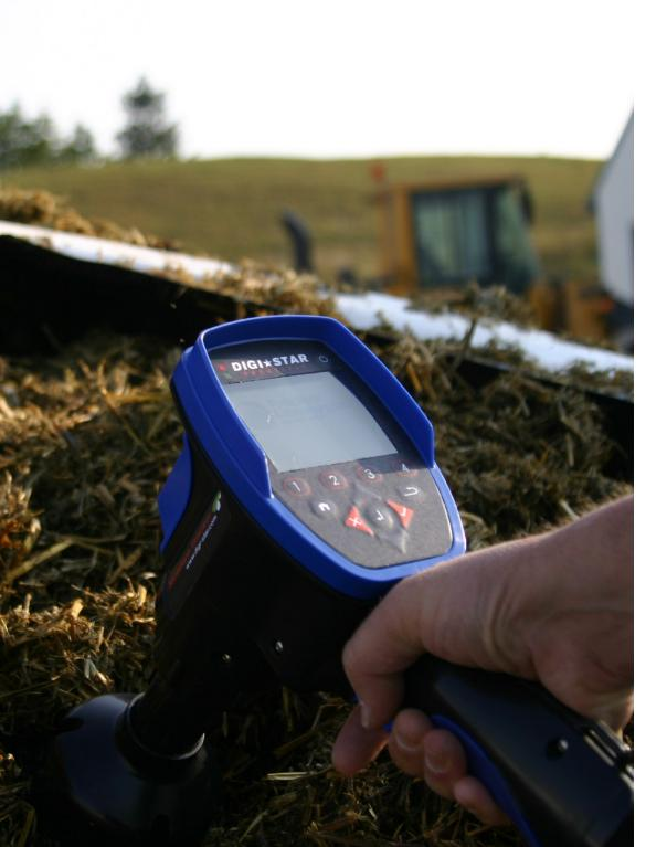
With Moisture Tracker™ you receive quick results for your ingredients, forages or crops. From a simple series of trigger pulls, you can have instant and accurate readings of each moisture and dry matter content.
