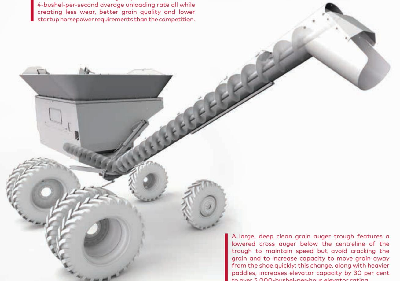
A large, deep clean grain auger trough features a lowered cross auger below the centreline of the trough to maintain speed but avoid cracking the grain and to increase capacity to move grain away from the shoe quickly; this change, along with heavier paddles, increases elevator capacity by 30 per cent to over 5,000-bushel-per-hour elevator rating.
