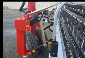
PARALLEL LINKAGE TORSION BASKET SUSPENSION
