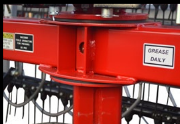
HEAVY-DUTY BASKET PIVOT w/ UHMW SHIMS -SHEAR BOLT PROTECTED
