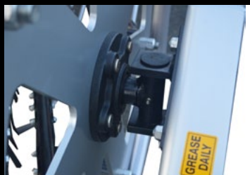
SELF-ALIGNING IDLER HUBS
