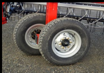
OFFSET DUAL WHEELS FOR MORE STABILITY
