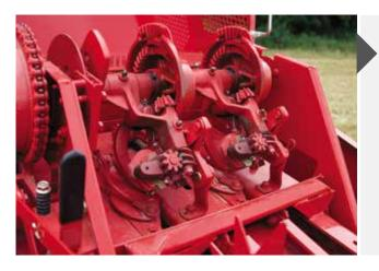
The Hesston design of knotters are built to operate reliably season after season, with minimum fuss or maintenance. Their rugged design guarantees excellent reliability bale after bale, whether using high quality plastic or sisal twine.
