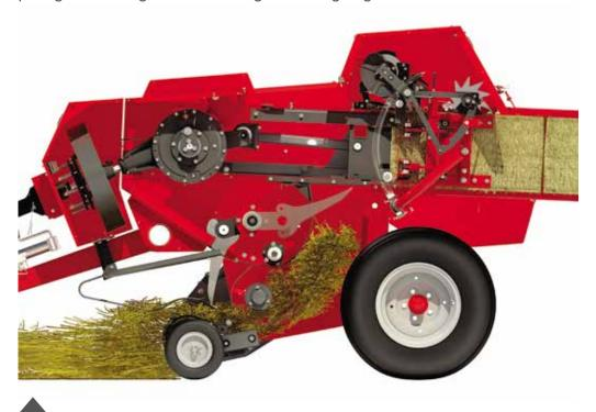
Crop is moved directly from the pick-up into a pre-forming chamber.
