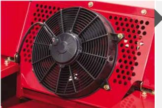
An electric knotter fan is fitted as standard to the MF1840 and ensures the knotter are kept clean and free from any debris build up during operation.
